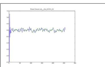
Fig1. Plot of closure phase of ALMA. For a point source, they must be zero phases theoretically. Variation from zero means the stability of interferometer system.
